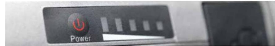
g. There are 5 active LED's on the battery. Push POWER to check the remaining capacity.
